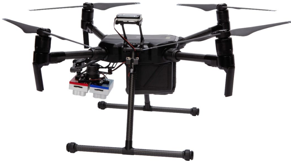
Fully connected Dual Camera Configuration on a DJI M200
