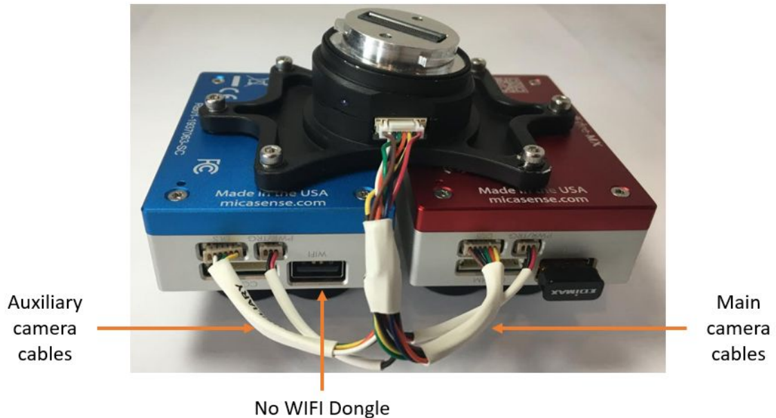
Connection between Dual Camera System Mount, RedEdge-MX and RedEdge-MX Blue
